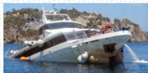
Yacht salvage using Salvage Pontoons 2,000 lbs. and Salvage Pontoons 20,000 lbs. Photo credit: Orca Commercial Diving, Italy.
