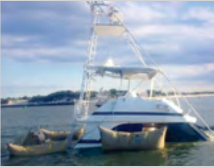
60 ft Yacht salvage using EFB-4000's and EFB-6000's. Photo Credit: Sea Tow Delmarva - Pennsylvania, USA
