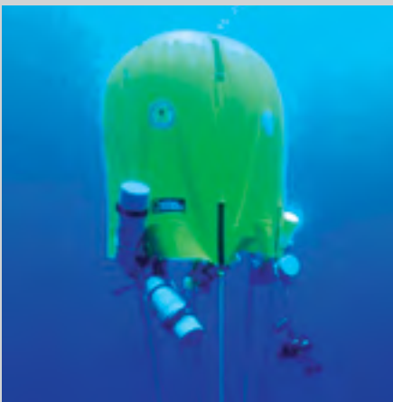
Custom inflatable underwater decompression habitat used by Michael Lombardi with National Geographic
