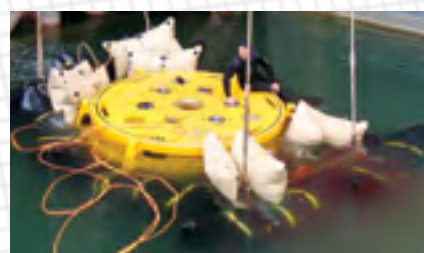
Lowering instrumentation using Enclosed Flotation Bags 500 lbs. and Enclosed Flotation Bags 6,000 lbs.
