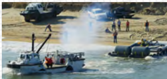
Salvage Pontoons 4,000 lbs. being used on an ocean wave energy system.
