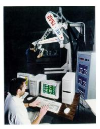
**SPDM Testbed Manipulator**
