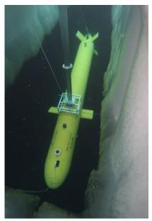
In 2007 ISE began work on the Swimmer project for Cybernetix S.A. of Marseille, France and Total. We designed a hybrid AUV system for work in deep oil fields. It comprises a shuttle AUV that carries and deploys a lightweight electric inspection and intervention ROV.
